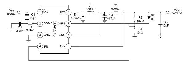
Figure 1. Application Circuit for 5V/1.5A Output
