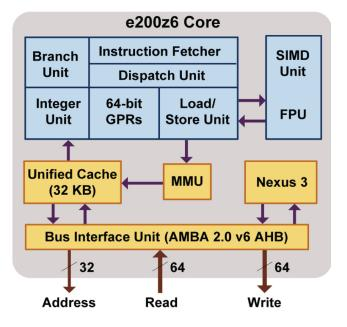
The z6 core is the high-end member of the e200 core family and offers the following features:
